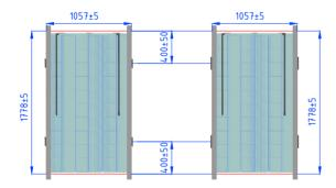
\*\*\*When a module is installed in portrait orientation on the pitched roof which has >45° slope, additional hook in the bottom of the module is required
